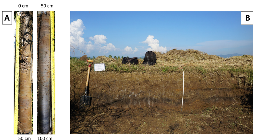
Figure 1. (A) Example of the stratigraphic successions found in the site of interest. (B) Outcrop found in a man-made drainage channel. Both images show black layers that potentially might be indicative of a buried soil caused by coseismic subsidence.
