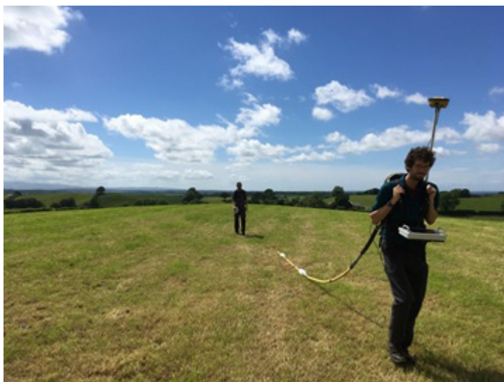
Figure 1. Collection of a survey line across a flat-topped hill using the GPR 100 MHz antenna.
