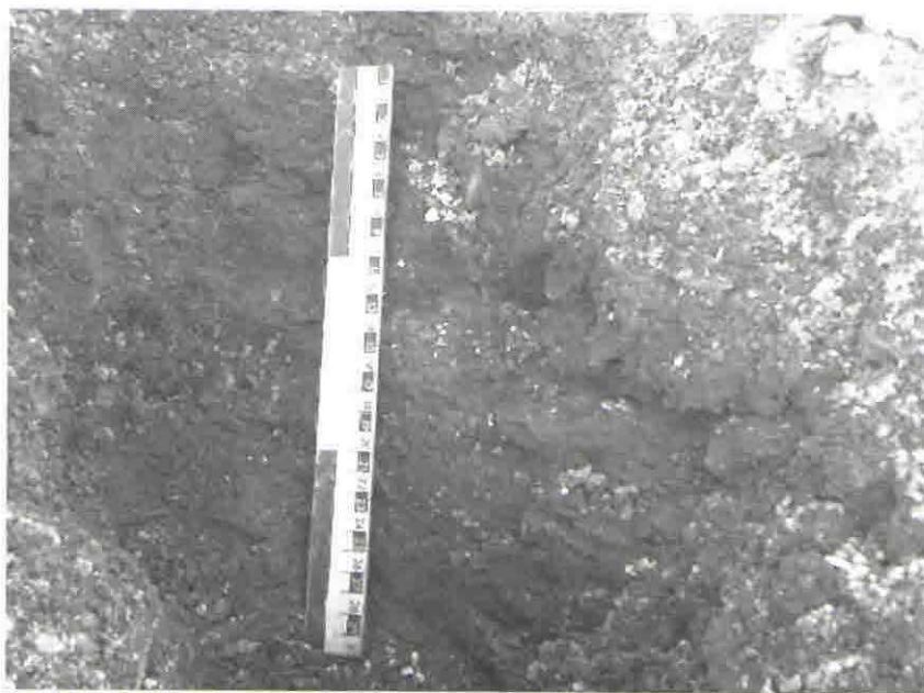
Figure 1. Thirty centimeters of cleared section from Breiða Windows location showing the presence of multiple black sand lenses and thin inter-bedded layer. Note the blocky structure.
