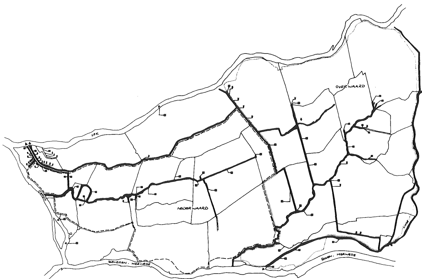
fig. 62. Drainage system of Overwaard and Nederwaard.
